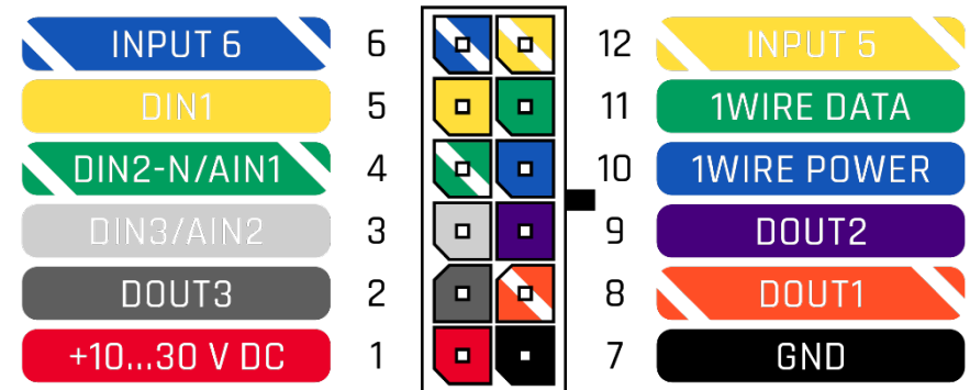
Figure 2 FMU130 2x6 socket pinout
