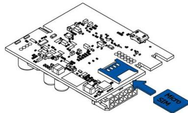
Figure 5 Micro-SIM card insert
