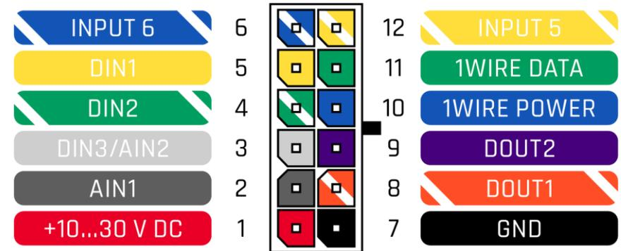
**Figure 2 FMB110 2x6 socket pinout**
