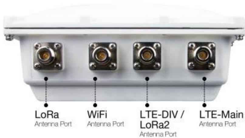
Figure 2 | Hardware Interfaces - Front
