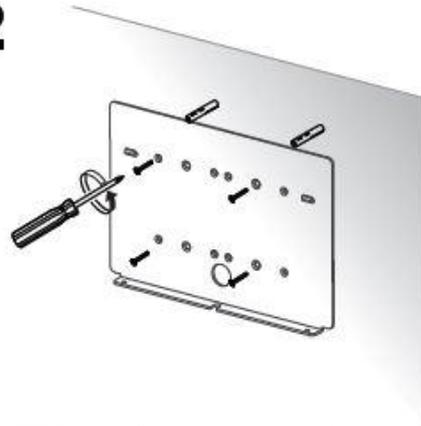
Install the wall mount kit on wall and screw in
