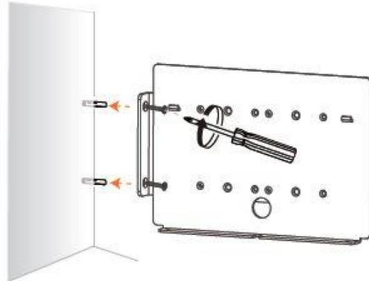
Screw the wall plug into the wall, then align the hole of the (L-shaped) small wall mount kit and then fasten in the screw.
