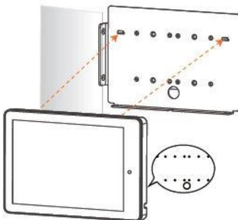
Hang up and align the wall mount kit with its hole
