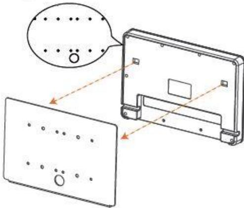
Hang up and align the wall mount kit with its hole
