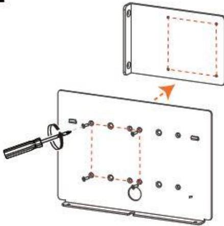
First align the small wall mount kit(L-shaped)) with the large wall mount kit at the screw hole and fasten the screw.
