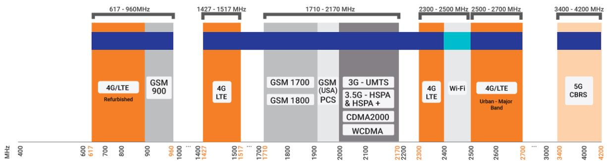
Indicates the LTE bands on which PUCK-1 works       Indicates the WI-FI bands on which PUCK-1 works
