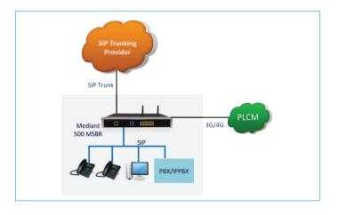
The Mediant 500 is equipped with an integrated Wi-Fi (802.11n) access point, as well as optional dynamic and static routing capabilities. The integral LAN switch supports up to four ports for IP phones or other devices. Customers can utilize up to four TDM voice channels and four PSTN ports with several combinations of analog and digital interfaces.
