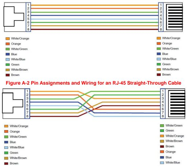
Figure A-3 Pin Assignments and Wiring for an RJ-45 Crossover Cable
