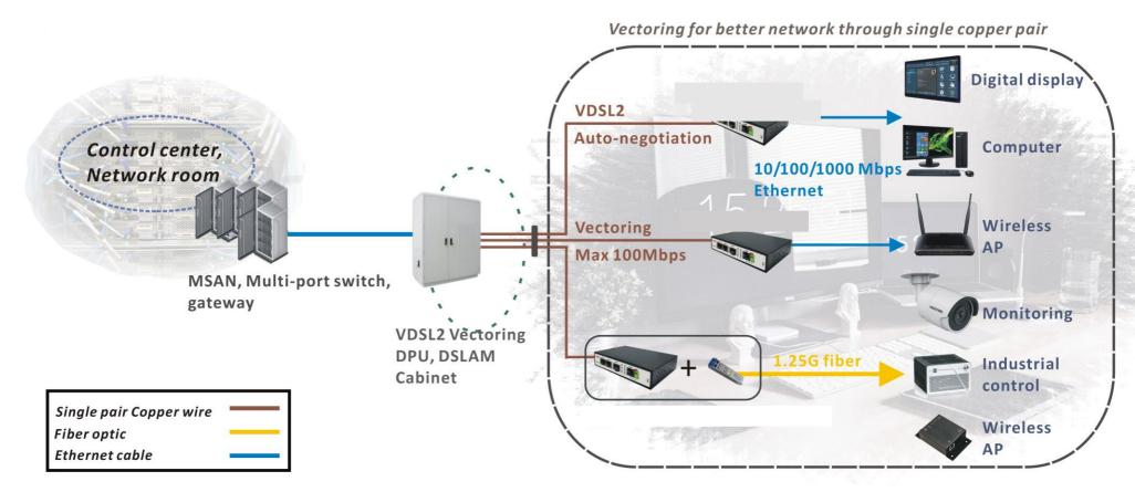
**Figure 2.2 Application Diagram**
