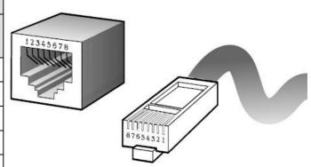
Figure A-1 Standard RJ-45 plug/connector
