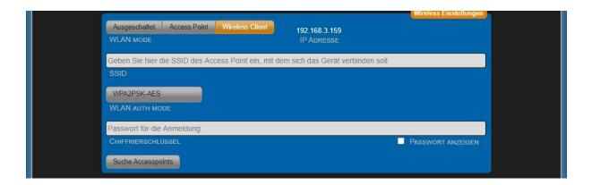
Select Wireless Client to connect the device to an existing network. Click Search Access Points to search for your WLAN network.
