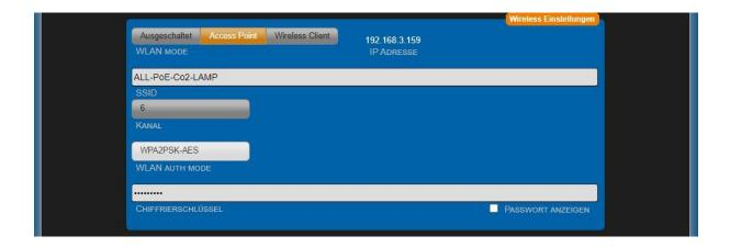
**SSID**: Here you can enter any network name. This name will be displayed when scanning the network.
