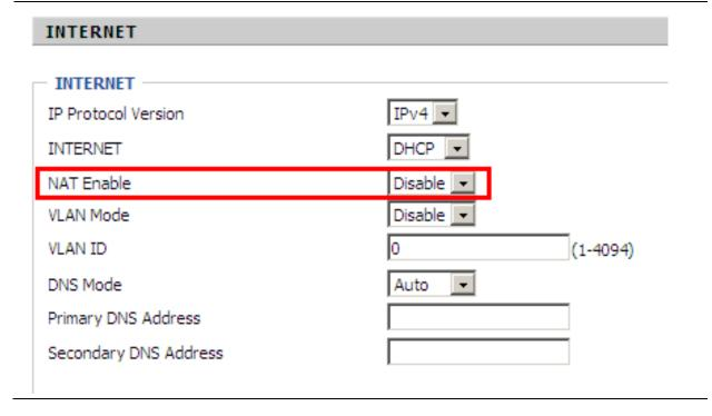
Step 2: Open Network-> WAN, Change NAT Enable to Disable. Save and Reboot. Now the device works in Bridge mode.
