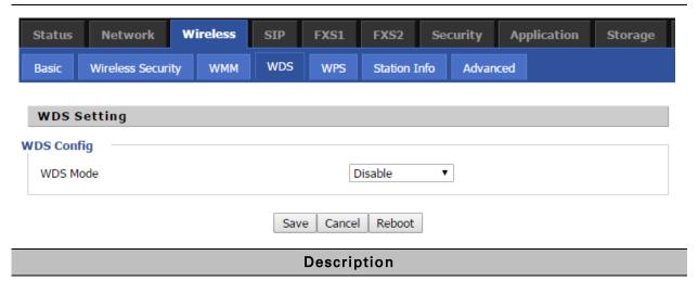
WDS stands for Wireless Distribution System, enabling WDS access points to be interconnected to expand a wireless network.
