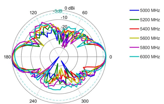
Azimuth Port 1 & 3: 2400 – 2500MHz | Azimuth Port 2 & 4: 5000 – 6000 MHz
