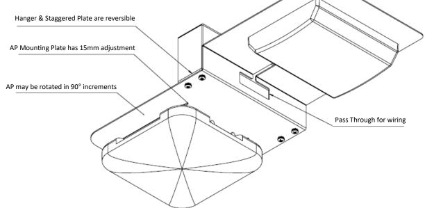
\*Range of beam sizes that the beam clamp mount can attach to:
