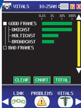
Vitals provides an indication of the operational condition of a network. A real time analysis of good and bad frames received is used to determine if the network is healthy or problems exist that may be affecting performance.
