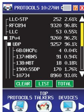
Lists all protocols detected with the total number of packets and the percentage of the total traffic. Certain protocols such as IPv4 and IPv6 can be expanded to show the sub-protocols.
