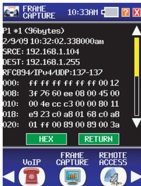
Capture up to 10,000 packets for analysis including packet size, source and destination IP address, time detected and packet type. User defined filters capture specific data needed to identify problems and monitor performance.
