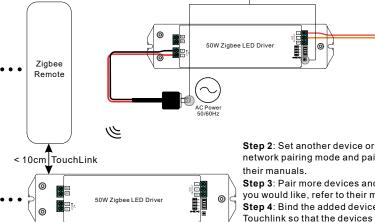
Step 2: Set another device or remote or touch panel into network pairing mode and pair to the network, refer to
