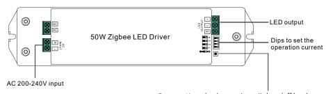
Program Key: short press to switch on/off load, press and hold down to increase/decrease light intensity
