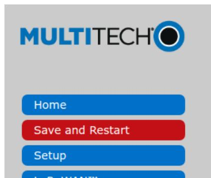
Figure : Restart button - MultiTech basestation
