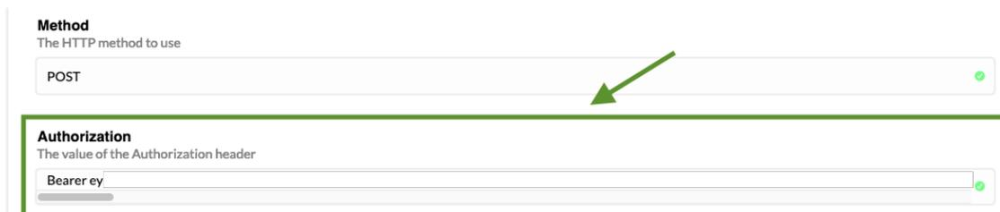
Figure : Step 4 - Authorization field on TTI HTTP integration
