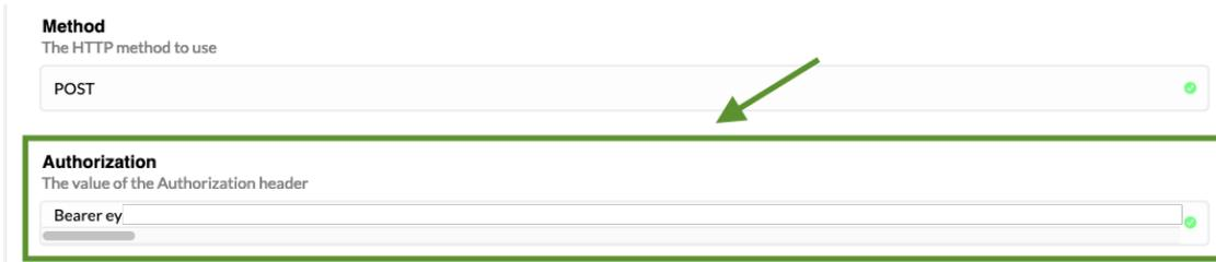
Figure : Step 4 - Authorization field on TTN HTTP integration
