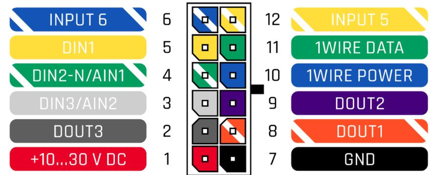
**Figure 2 FMM130 2x6 socket pinout**
