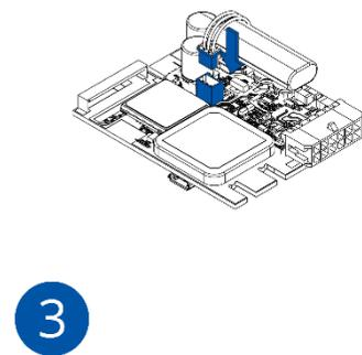
Figure 6 Battery connection
